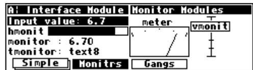
Each of the graphical control signal monitor modules has a control signal input and four *specifiers*: minimum, maximum, name and tag.
