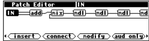
Insert an eq module by pressing the <insert> SOFT KEY, scrolling to the Filter group, and selecting eq. Press the SELECT key to actually insert the eq module.
