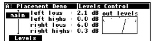
To achieve this arrangement, the modules' *userobject* outputs must be connected to the *menupage* module in exactly the order shown to the right:
