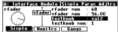
The choices appear in place of the %s in the menu statement. The 8 char name is only used if the module's *userobject* is connected to the head module. The control output reflects which selection is made. If the 1st selection is made the output will equal 0. If the 3rd selection is made, the output value will equal 2. Refer to the **Modules Section** for complete information.
