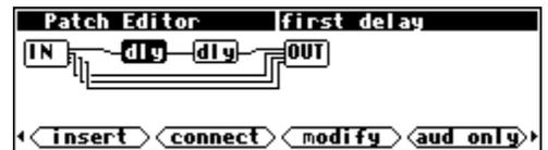
. . .and then press the <modify> SOFT KEY. On entry to the <modify> menu, the display shows the current KNOB mode (select or adjust), the name of the module, the module type, and the first three lines of module information.
