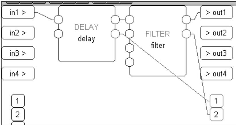
For example, consider the simple delay module connected to a filter module we started this chapter out with (again, as shown in *VSigfile*). Now that you've learned a little more, we've "unhidden" the control inputs for these modules (the unconnected ones on the left) and the *userobject* outputs (the ones on the lower right). As you can see, we've connected their *userobject* outputs to the *userobject* inputs on the head module (the disembodied "1" and "2" in the lower right corner).
