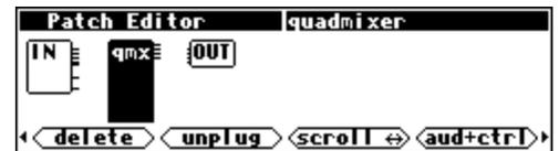
The screen will not move if there is no off-screen information in the direction that you are spinning the KNOB. Thus, in the case of a simple program such as the one shown to the right, selecting scroll motion up and down and then rotating the KNOB will cause no change.
