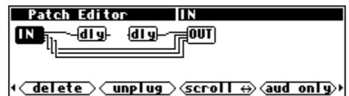
That's it. You've "unplugged" the input to the delay module.
