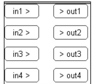
In the simplest of conceivable programs, the IN module's outputs are connected directly to the OUT module's inputs (this is the Thru' program in bank 0). Normally, other, optional modules are inserted in-between the IN and OUT modules.
