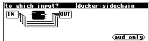
highlighted little line inside the OUT module. Rotate the KNOB (or use the LEFT or RIGHT CURSOR key) to select the ducker's sidechain input. As you move the highlighted little line between available inputs, the upper right-hand side of the display will show the currently selected input and the name of the module it resides on.
