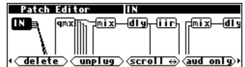
The <scroll> SOFT KEY changes to reflect current scroll mode, allowing you to scroll either horizontally or vertically.
