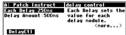
The menu page shown above is visible in the PARAMETER area. It is created with a menupage module, a knob module, a monitor module, and a textblock module (*we'll see how in a minute*).
