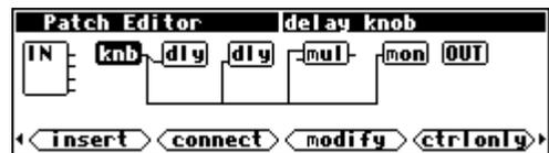
As an exercise, you could go to ctrlonly screen mode and bypass the mul module by connecting the knob (knb) to mon-i n (as shown to the right). That would make the Delay Amount parameter in the PARAMETER area show the correct delay value.
