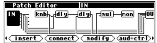
Go back to the PARAMETER area (by pressing and holding the PARAMETER key) to see how these modules and their connections in the Patch Editor area translate into parameters on a menu page. The monitor module creates the parameter Delay Amount that shows the actual delay, while the knob creates the parameter Each delay that sets the delay for each of the delay modules.
