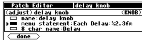
Now go to the PARAMETER area and see the difference that made to the display. Note the decimal value in the “Each Delay” parameter. It used to read 250. Now it reads 250.000. *Contain yourself . .*
