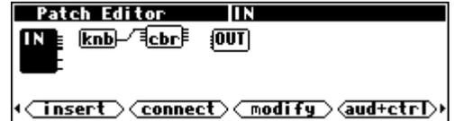
Additionally, the knob module's *userobject* output is connected to the head module so that the knob module's parameter shows up in the PARAMETER area as shown to the right.
