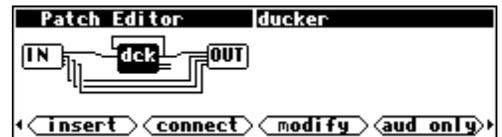
Now the compressor will be heard on the first "channel" of the DSP running the program, while the remaining three "channels" go uncompressed. Press and hold the PARAMETER key to see the ducker module's menu page.
