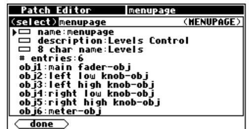
To create a menu page such as the one shown, the programmer inserts the six “parameter” modules and the *menupage* module using the <insert> SOFT KEY and then uses the <modify> SOFT KEY on the *menupage* module. The # entries is first set to the desired number (six) and then the obj entries are adjusted, one at a time, to connect the *userobject* outputs to the *menupage* module.
