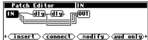
The current program now has a single delay module between IN:i n1 and OUT:out1, a del ay module that has an input but no output, and straight paths between the remaining DSP "channels." Note that the signal that was *previously* connected to OUT:out1 has been automatically disconnected. See Notes below.
