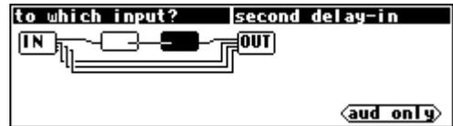
Although the <aud only> SOFT KEY is presented, pressing it in this case will *not* allow connections to anything that *isn't* an audio or mod input. This is because we've already selected an *audio* output, and you can't connect an *audio* output to anything but an *audio* or *mod* input. Feel free to press the <aud only> SOFT KEY, and you'll see what we mean.
