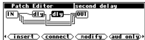
You should now be able to connect IN:i n2 to second del ay:i n. Then connect second del ay:out to OUT:out2. The screen to the right is what you should end up with. This "patch" has a delay module in each "channel" of audio.
