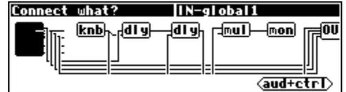
Using the CURSOR keys, select the output of the leftmost dly module. You'll know you have the correct output when the upper right of the display reads first delay-out. When the screen looks like the one shown to the right, press the SELECT key.
