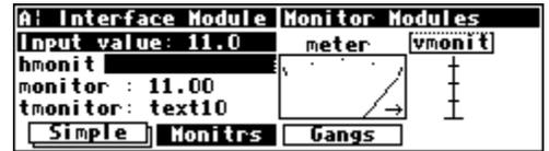
The vmonitor module creates a graphic that is one sixth of a screen width and four lines high. The hmonitor module creates a graphic that is one half of a screen width and one line high. The meter module creates a graphic that is one quarter of a screen width and four lines high. *Form over function...*
