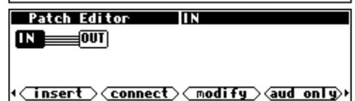
To start creating the compressor, insert a ducker module. Press the <insert> SOFT KEY. You will get a list of things to insert.
