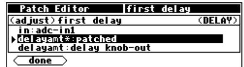
If "autoknob" is chosen (as in the example to the right), the next line of the menu will show the "autoknob's" PARAMETER area menu statement along with the current value of the control input (first delay: 101.00 ms in the example to the right). More on this below under "Autoknob." . .
