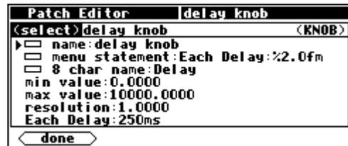
As another wee exercise, load the program Patch Instruct from the “Programming” bank, go to the Patch Editor area, change the screen mode to aud+ctrl, and highlight the knb module. Then use the <modify> SOFT KEY to change the min value and max value to set different limits as shown to the right.
