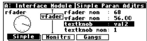
The choices appear in place of the %s in the menu statement. The 8 char name is only used if the module's *userobject* is connected to the head module. The control output reflects which selection is made. If the 1st selection is made the output will equal 0. If the 3rd selection is made, the output value will equal 2. Refer to the **Modules Section** for complete information.
