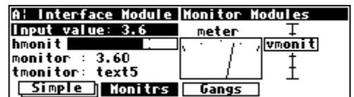
The monitor module is a mirror image of the knob module; it displays the decimal value of its control input. The format for the display is set using the text and %f format described earlier.
