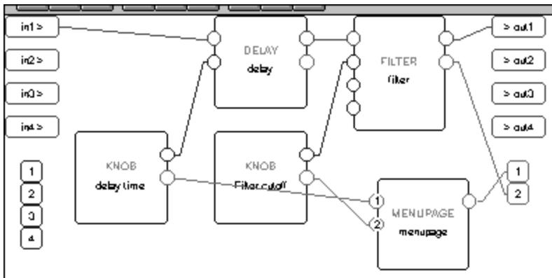
For example, we could utilize two knob modules and a menupage module in the program we've been working on. One knob module will take over the delay time control input on the delay module. The second knob module will take over the frequency control input on the filter module. The *userobjects* of both knob modules are connected to the menupage module, which is in turn connected to the head module.
