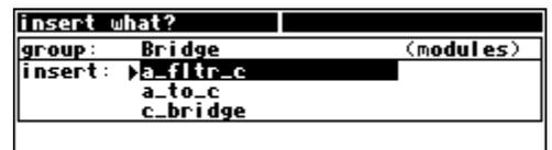
Note that modules do not, strictly speaking, have to be in any particular order because connections can run in either direction. However, the programmer should be aware that every instance of reverse signal flow will add a four sample delay to the process. In some cases, such as where a preset has multiple signal paths, such delays can cause objectionable "phasing," or other artefacts.
