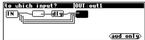
After you've experimented, set the screen mode back to aud only, select out1 on the OUT module, and press the SELECT key.
