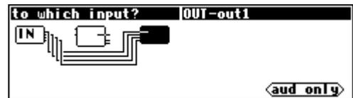
Notice that the output we selected is still identified by a little line inside its module box, but the box itself is not highlighted. The little line tells us what we're connecting *from*. The editor is now asking what input we would like our previously selected output connected *to*. The currently selected input is shown as a
