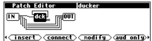
The last thing we need to do is connect the OUT module to the ducker so that we can hear what the compressor sounds like. Press the <connect> SOFT KEY and then the SELECT key to select the ducker's output. Press the SELECT key again to connect that to the OUT's output 1.
