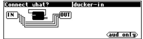
Press the SELECT key to actually select the ducker's main input. Now we need to select something to connect the ducker's main input to. As luck would have it, the IN module's input 1 is the currently selected candidate.
