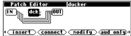
Note that the IN and OUT modules are still connected to each other, just as they were. Audio is still passing through the DSP running Thru unchanged!
