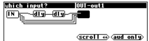
Use the LEFT CURSOR key to select the input for the second delay module.
