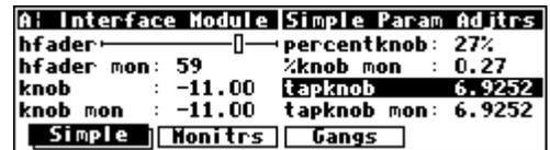
The tapknob module creates a tapered (non-linear) control that has a “selectable” number of steps (instead of the usual resolution parameter) and a “selectable” taper waveform. The greater the taper *specifier*, the more non-linear the parameter response. Refer to the **Modules Section** for complete information.
