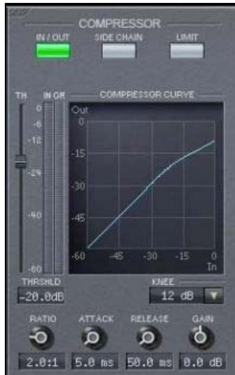
Figure 4 E-Channel Compressor module
