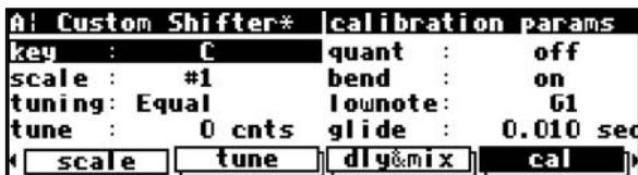
The **Key** and **Scale** parameters are useful for MIDI control. You'll be able to transpose the current selected scale to any of 12 keys and you can recall any of up to 12 internally set and stored scales.
