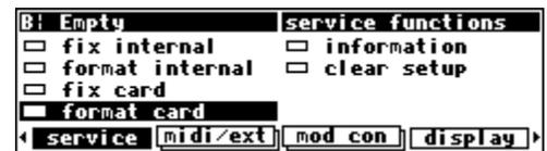
Highlight format card and press the SELECT key. Pressing the <yes> SOFT KEY will erase the contents of the Memory Card and reformat it. Press the <no> SOFT KEY to abort.
