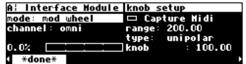
If omni is set to off on the `[midi]` menu page in the SETUP area, then the second parameter on the screen, channel, selects which MIDI channel the MIDI message will be accepted on (relative to the base channel found on the `[midi]` menu page in the SETUP area). If the value of base + x is greater than 16, the result "wraps" around. For example, if base channel were set to 10, and channel were set to base + 12, the *actual* MIDI channel used would be
