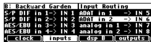
Now, we need to assign the S/P DIF, AES/EBU, and ADAT inputs to the first six inputs of DSP A. Do this at the **DSP A** menu page in the **SETUP** area. Strictly speaking, assigning silence (-----) to the last two inputs isn't really necessary since we don't plan to use those outputs ...
