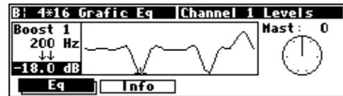
Pressing the DOWN CURSOR key on the screen above would move the cursor from the graphic interface to the Mast parameter.
