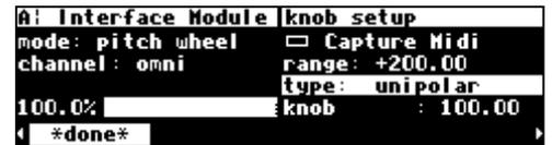
Adjust the value of the parameter being modulated to remedy this situation (*see further examples below*). In this case you're going to manually change the value of knob to 0 while the pitch wheel is idle (at 50%).
