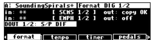
Note: The digital inputs 1/2 need not be assigned to the same protocol as the digital outputs 1/2. In other words, digital inputs 1/2 can be received at the AES/EBU 1/2 input jack and digital outputs 1/2 can be sent via the S/P DIF protocol. Or *vice-versa*.
