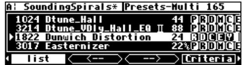
**Sort By Effects** sorts programs based on their fundamental effects types. As shown here, all of these programs use pitch shifters (**P**), delays (**D**), and modulators (**M**). If you were to use the **KNOB** to scroll up or down, you would find other groupings. Use the left and right **CURSOR** keys to skip from grouping to grouping (e.g. from programs that use **PDM** to programs that use **RDM** to programs that use **PRDM** and so on).
