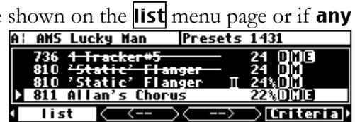
Similarly, some programs come in two versions: a monolithic version for 88/96k operation, and a single machine version for 44/48k operation. Normally only the relevant one of these is visible, but if **Show** is set to **any**, both of these can be seen, as shown by 'Static' Flanger in the screen above.
