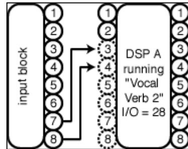
To the right, we have another bad scene. The program "Big Voice" has an "I/O Identifier" of "22." That means that only DSP outputs 1 and 2 are live. Outputs 3 through 8 are dead, but in the block diagram to the right, it is these dead outputs that are being used. Again, you won't hurt the H8000 by hooking things up this way, but you won't pass audio!
