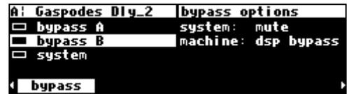
To "un"-bypass a DSP, press its bypass x field again. Its corresponding Bypass Status LED will grow dark . . .
