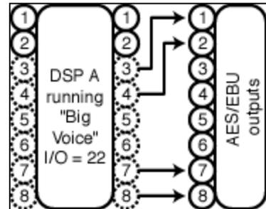
Of course, making a connection to a dead input or output is not *necessarily* a bad thing. You can make "dead connections" as long as you don't fool yourself into thinking that they're actually passing signals.
