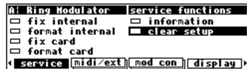
Highlight **clear setup** and press the **SELECT** key. Pressing the <yes> **SOFT KEY** will replace current parameter values with the "factory defaults." *Unless you saved your setup before pressing <yes>, it will disintegrate into digital dust (see [Storing and Loading Setups](#) on page 93).* Press the <no> **SOFT KEY** to abort. If the H8000 ever gets "buggy," try using **clear setup** before you do anything more "drastic."
