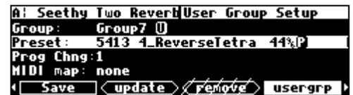
This line shows the programs according to the Search and Sort options on the **Criteria** page. The wheel or keypad can be used to move through them in the same way as on the **list** screen.
