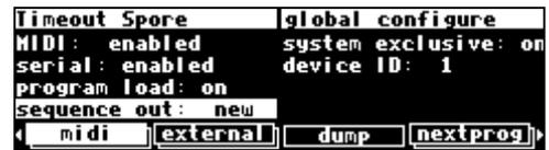
Simply play back the recorded MIDI sequence at the H8000's MIDI In, and you will see the changes you recorded "played" by the sequencer (*assuming MIDI is enabled, system exclusive is on, the programs that were loaded when the sequence was recorded are loaded during playback on their respective DSPs, and the device ID set during recording is set during playback*).
