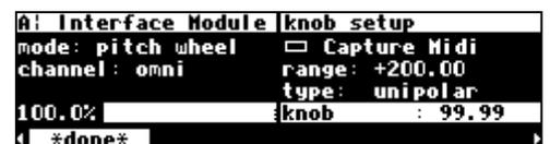
Note: It is also possible to set range to a negative value. Doing so allows the value of the parameter being modulated to *decrease* while the external controller is *increasing*
