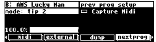
On the **nextprog** menu page in the SETUP area, you'll find an external trigger menu page. The "top" menu page selects a trigger to load the next program, and the "bottom" menu page selects a trigger to load the previous program (press the **nextprog** SOFT KEY to toggle between the two).
