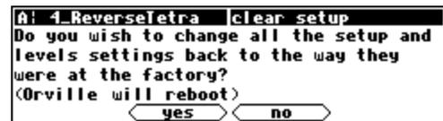
Alternatively, you can clear the internal setup by holding down the **SETUP** key during startup.
