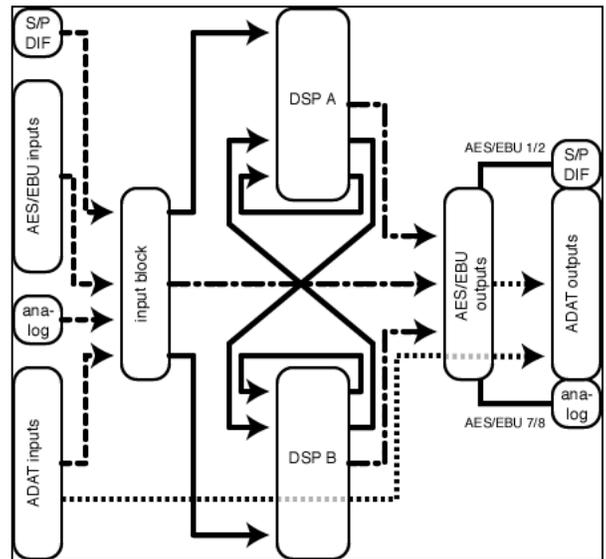
Next, "sources" are assigned to the main AES/EBU outputs (dot-dash arrows in the diagram). Again, the available sources are:
