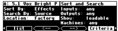
The fourth and fifth parameters, **Inputs** and **Outputs**, filter which programs are shown on the **list** menu page based on how many inputs or outputs they use. Your choices are **any** (any number of i/o's), **stereo** (2 or 3 i/o's), **quad&2+2** (4 or 5 i/o's), **5.1** (6 or 7 i/o's), and **octal** (8 i/o's). This allows you to only display programs suitable for your application, i.e. if you are working in **5.1** you may not want to be bothered with **stereo** effects, and *vice-versa*.
