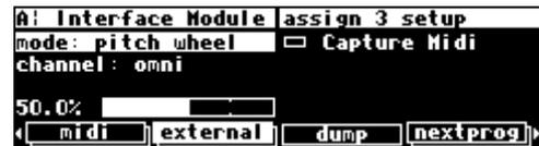
Now, when you move the pitch wheel both S/P DIF in 1 and A OUT4 Wet/Dry are modulated!
