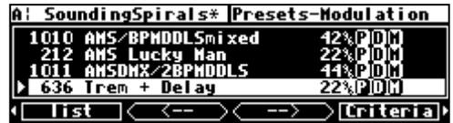
The second parameter, **Search By**, causes the **< --** and **-- >** trigger **SOFT KEYS** to perform searches using different criteria. The default value, **All**, doesn't perform any search at all. Every program in the H8000 is listed on the **list** menu page in the order defined by **Sort By**.
