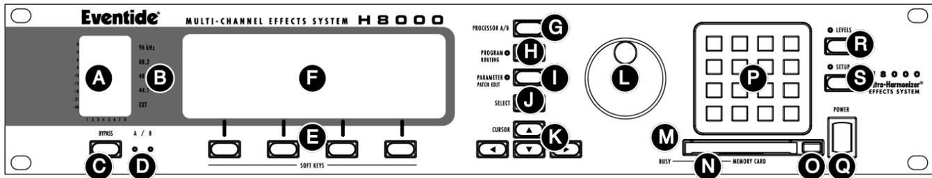
**A) Level Meters** These measure the eight signals selected for input, DSP A's eight inputs, DSP B's eight inputs, DSP A's eight outputs, DSP B's eight outputs, or the eight AES/EBU outputs (from which all of the other outputs are derived).
