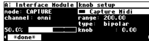
The next type of MIDI message received by the H8000 will be used for the mode parameter, and the MIDI channel that it is received on will be used for the channel parameter. Of course, if you are in omni mode, the channel parameter will remain omni regardless of what channel the message is received on. *To exit "Capture" mode without "capturing" just press the SELECT key again.*
