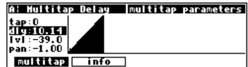
Use the LEFT and RIGHT CURSOR keys to select the particular tap for which you're adjusting parameters. The graphic to the right of the parameters represents the delay position and level of every tap in the bunch.
