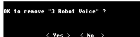
Factory presets are distinguished from your saved presets by the lack of a "U" at the right-hand side of the screen. You can't delete any of the factory presets. That's why <remove> is scratched out when a factory program is highlighted on the **list** menu page.
