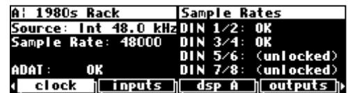
If you use the H8000's internal clock, be sure that the digital devices that are connected to it derive their clock signals from the H8000. If you are unable to synchronize any of the AES/EBU inputs or the S/P DIF input, turn on the H8000's sample rate conversion (SRC) algorithm on the "second" and "third" **clock** menu pages in the SETUP area. The H8000 does not have sample rate conversion for the ADAT inputs.
