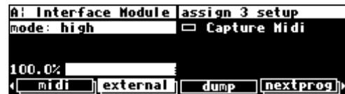
You can set mode to anything you like; we're going to set it to pitch wheel on channel omni (*the omni parameter on the [midi] menu page in the SETUP area needs to be set to off in order to assign a specific channel*).
