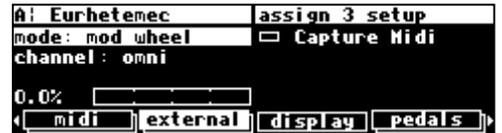
controller mod wheel has been selected to "fill" the "placeholder" *assign 3*.
