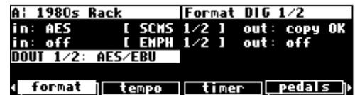
To be clear, the signal assigned to digital outputs 1/2 will come out *both* the AES/EBU 1/2 port and the S/P DIF port regardless of your choice. Your choice simply defines the digital *protocol* the signal will use. Both AES/EBU 1/2 and S/P DIF use the *same* protocol as defined on this menu page. Use the professional (AES/EBU) protocol unless you have a compelling reason to do otherwise ... you are a professional, aren't you? Eventide does not recommend the use of S/P DIF above 48kHz sampling.
