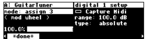
The `external` menu page is "stacked." Press the `external` SOFT KEY repeatedly to cycle through menu pages for *assign 1*, *assign 2*, *assign 3*, ..., *assign 8*, *trig 1*, and *trig 2*. These menu pages behave just like those that were discussed in [External Modulation and Trigger Menu Pages](#) on page 64, except that there is no range parameter.
