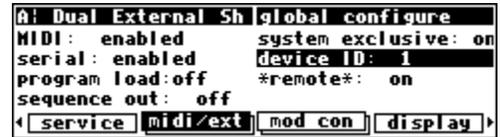
Now, changes made on the "master" are echoed on the "slave." Be sure to leave sequence out to off on the "slave" or MIDI "feedback" will lock up the H8000s in a very bad sort of way.
