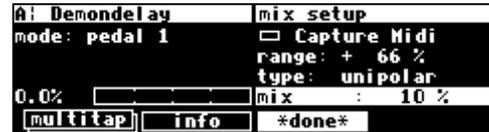
When type is set to unipolar and the external controller is all the way up, the parameter will take on a value determined by the *origin* and the range. Here 10% plus 66% = 76 %.
