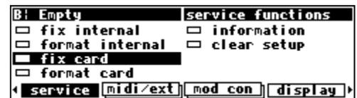
Highlight fix card and press the SELECT key. Press the <yes> SOFT KEY to force the new checksum result to be saved. If data is in fact corrupted, this will not fix it. Press the <no> SOFT KEY to abort.
