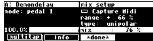
When type is set to bipolar, the parameter takes on the value of the *origin* when the external controller is halfway up (or halfway down if you're a pessimist).
