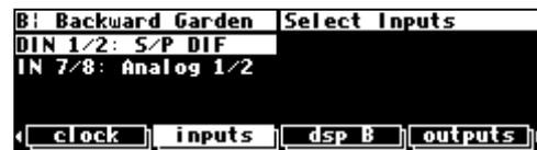
Then we need to make sure the appropriate inputs are selected at the input block. Do this at the "top" **inputs** menu page in the **SETUP** area. We're not planning on using input 8 so it doesn't really matter what gets assigned there!
