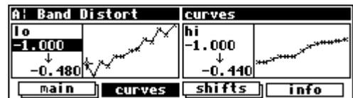
We could get a little wackier. How about making an input amplitude of 0.667 result in an output amplitude of -0.5? No sweat. By making the input amplitude radically different from the output amplitude, you can obtain a "garbage compactor" distortion.
